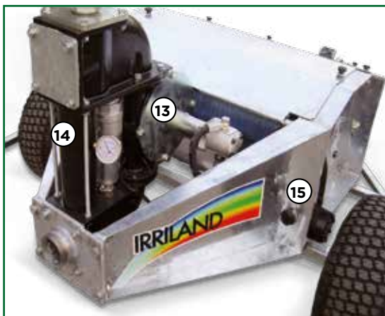
13. Turbina e pompa idraulica Turbine and hydraulic pump Turbina y bomba hidraulica Turbine und Hydraulikpumpe Turbine et pompe hydraulique
